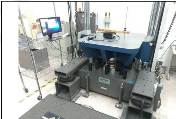
13. Mechanical Shock Test: -Z axis
